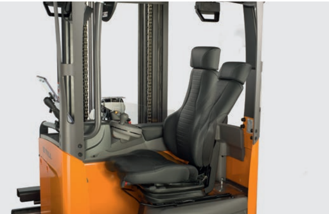
Comfortable tilt seat optimises upward visibility
