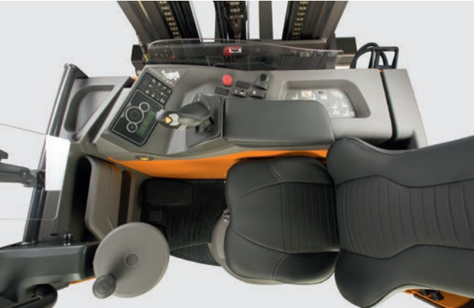
Adjustable driver's cab with numerous storage compartments
